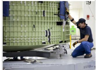
Image above: Inside the Operations and Checkout Building high bay, a technician attaches a crane to the Orion Exploration Flight Test 1 crew module so that it can be moved.
