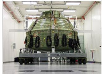
Image above: The Orion Exploration Flight Test 1 crew module undergoes proof pressure testing at the Operations and Checkout Building.
