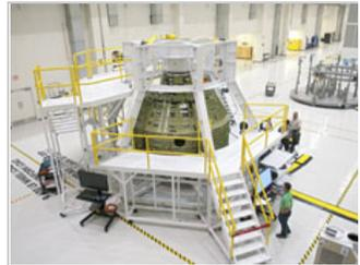
Image above: Inside the Operations and Checkout Building, a birdcage tool along with work platforms surround the Orion Exploration Flight Test 1 crew module.
